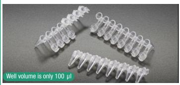
This flat cap low profile model has a volume of only 100 µl per tube, for a total of 8 tubes.
