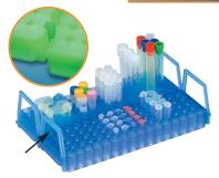
Units can be firmly anchored laterally to one another, thanks to special anchor pins supplied with each rack.
